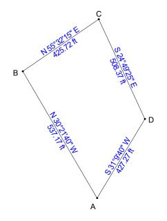
What is the radius of an arc tangent to sides AB, BC, and CD of the traverse? Determine to 0.01 ft.
