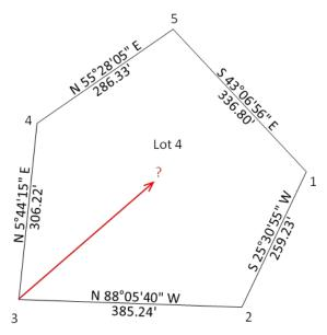
What is are the length (to 0.01 ft) and bearing (to 01") of a line from point 3 that divides Lot 4 into two equal areas?
