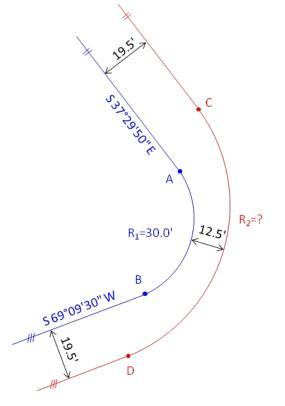
What is the maximum radius,  $R_2$ , of the tangent arc CD so that it comes no closer than 12.5 ft to tangent arc AB? Determine t nearest 0.01 ft.
